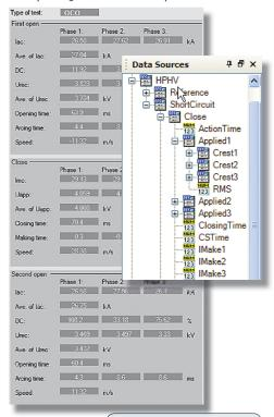
Major output results of short circuit 3 phase and Output results in the Data Sources.
