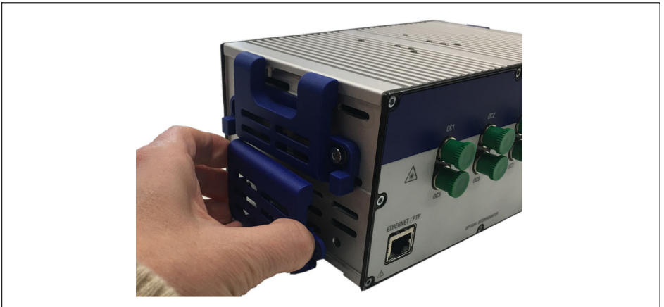
Fig. 3.14 Removing the bottom side cover
