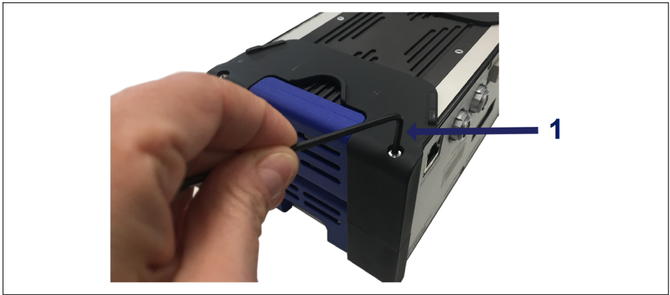
Fig. 3.12 Removing case protection
