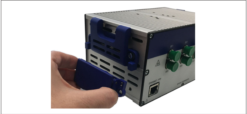
Fig. 3.15 Mounting the CASECLIP
