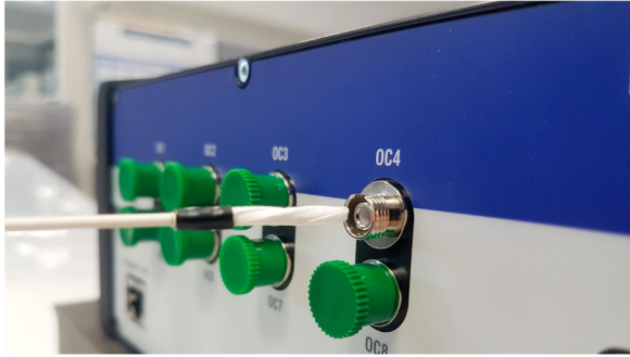
Fig. 3.28 Cleaning the connector adapter of the interrogator
