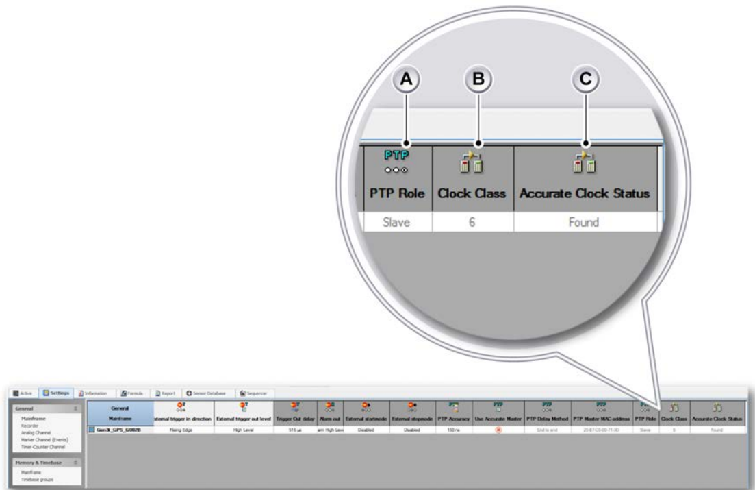
Figure 14.18: PTP synchronization status
