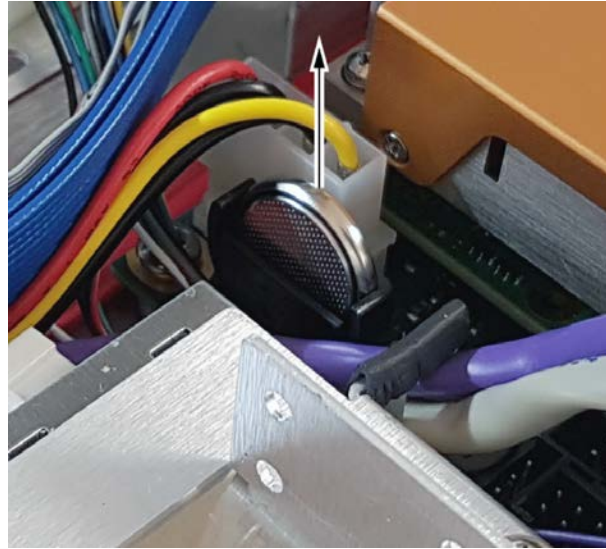
Figure 4.3: Remove battery (CPU section)
